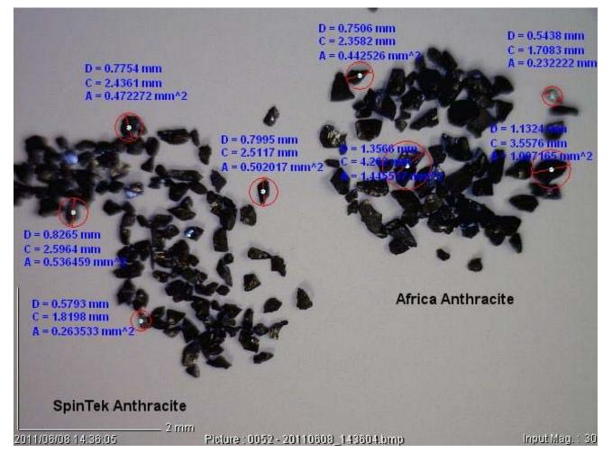
Photo Magnification Showing tight distribution and particle size of SpinTek Anthracite
