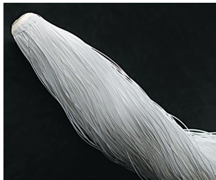
Hollow fiber membranes can be assembled into bundles
