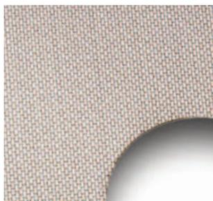
Closeup showing woven wire mesh
