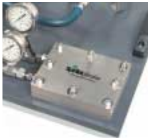
Close-up of quick-change membrane unit
