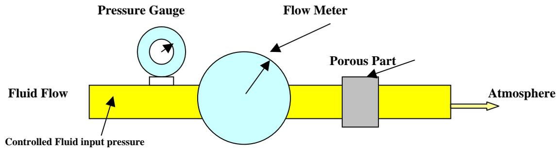
Parts used in time delay applications may be tested for elapsed time under simulated working conditions rather than in steady state flow.
