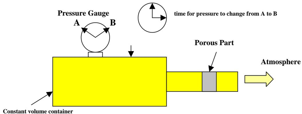
Several International Standards have been developed for testing permeable sintered metal materials:
