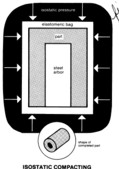
Isostatic Compacting is a process by which pressure is applied uniformly to a deformable container holding the metal powder to be compacted. This technique is especially useful in the manufacturing of parts having a large length-to-diameter ratio.
