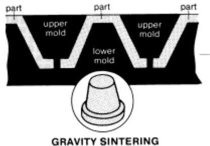
Part tolerance should be as liberal as can be allowed for the following reason: although I.D.'s tend to be predictable, because the material usually shrinks to the core during sintering, the O.D. will vary somewhat from piece to piece depending on size, shape, material, density of “fill” etc. Hence, design tolerances of  $\pm$  two percent should be used as a guide in gravity sintering. When required, closer tolerances can be held by a sizing operation.
