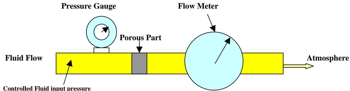
When it is difficult to collect all of the gas from a P/M part (for example, a long tube), the flow meter may be placed in the line before the P/M part. In this case the flow meter readings must be corrected for the pressure.
