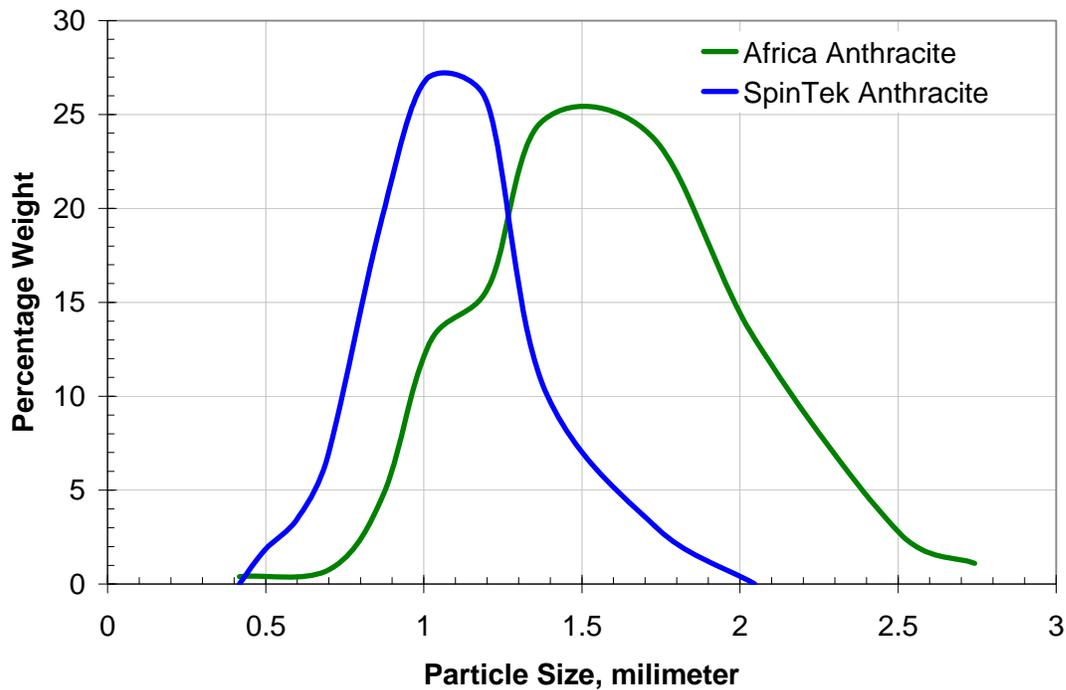
The varying distribution and particle size of the African Anthracite versus the tight distribution and particle sizing of the SpinTek Anthracite can be easily seen in the visual below:
