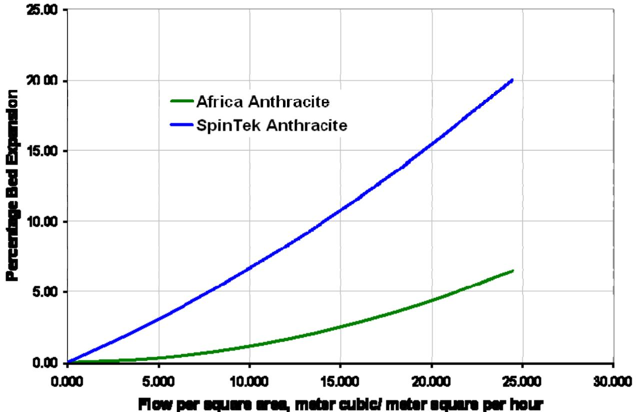
As can be seen the SpinTek anthracite meets the 15% expansion when the filter is backwashed at 20 m<sup>3</sup>/hr-m<sup>2</sup> whereas the Africa anthracite never meets the targeted backwash value.
