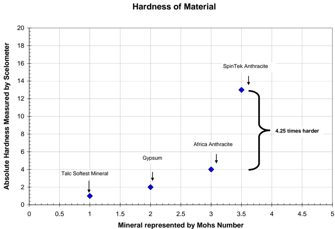
The hardness is important as the harder the anthracite is the less fines and better flow distribution that will be obtained.
