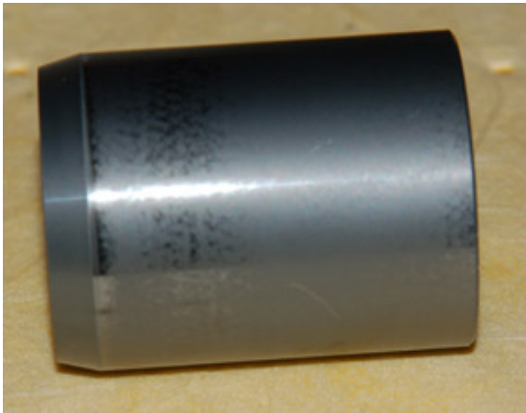
Figure 18. Shaft Bushing after 143 ½ hours of Operation
