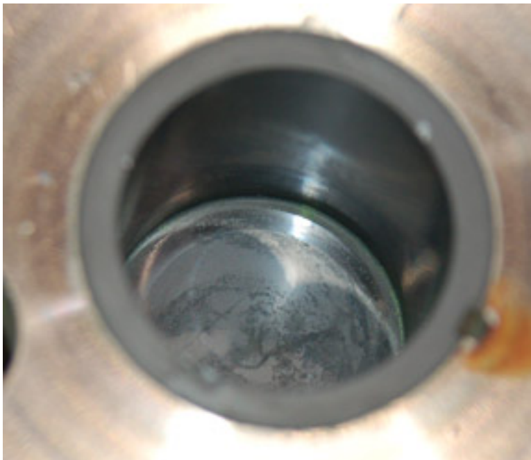
Figure 19. Receiver Bushing after 143 ½ hours of Operation
